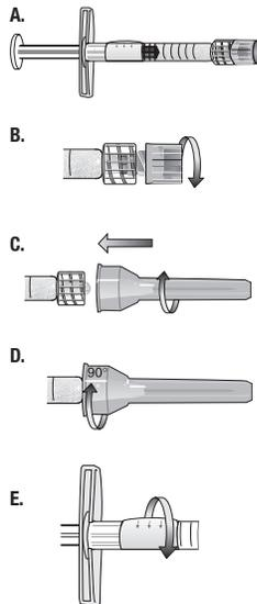
ASSEMBLY OF 29 G NEEDLE TO SYRINGE
